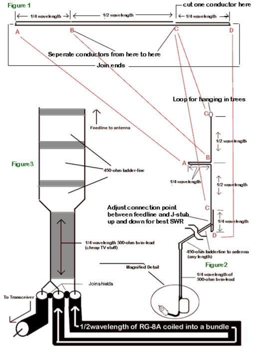
Don't forget to calculate the velocity factors of the transmission and phasing lines
