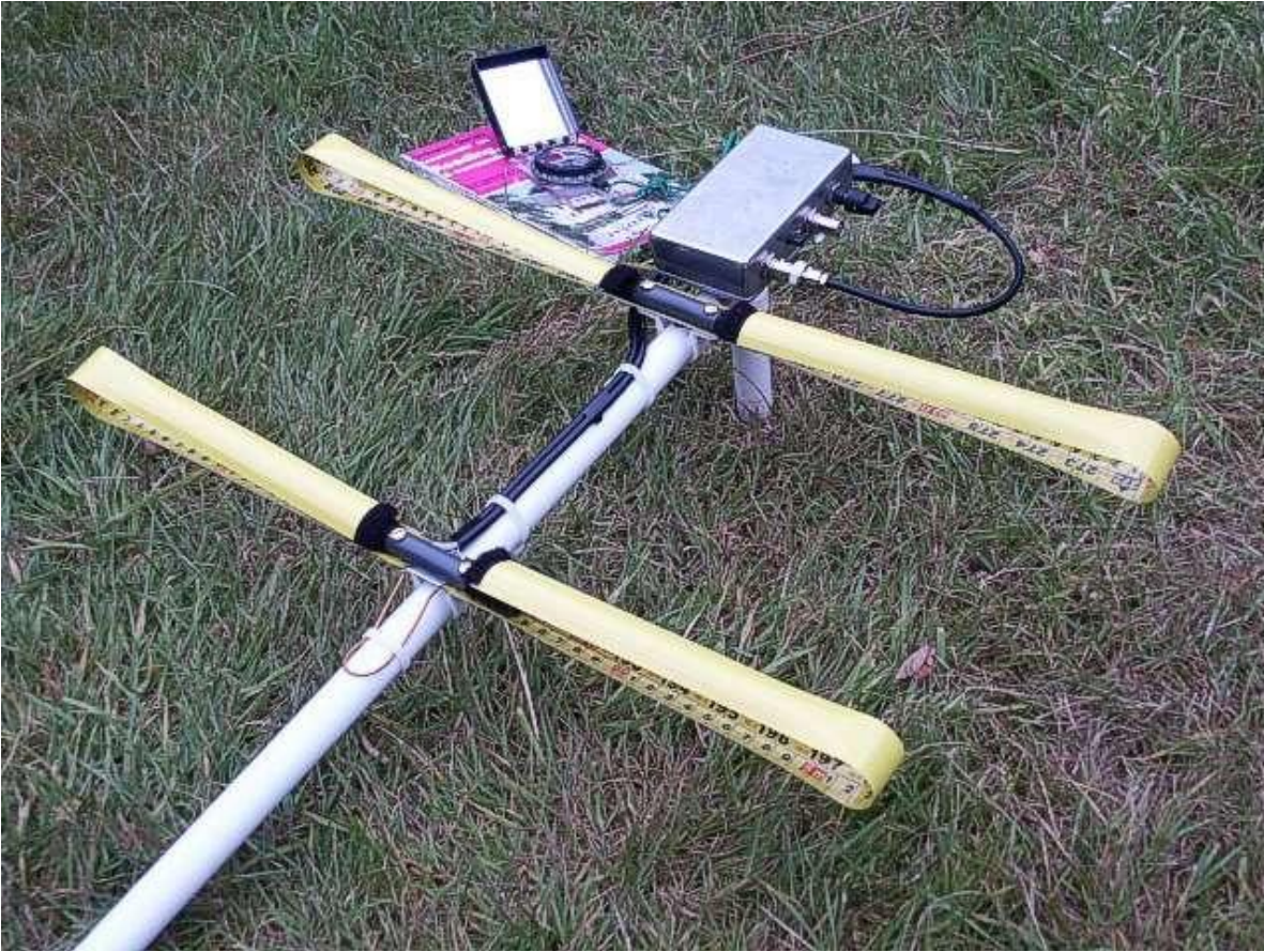
View showing the use of Velcro on the element ends to fold the elements.
