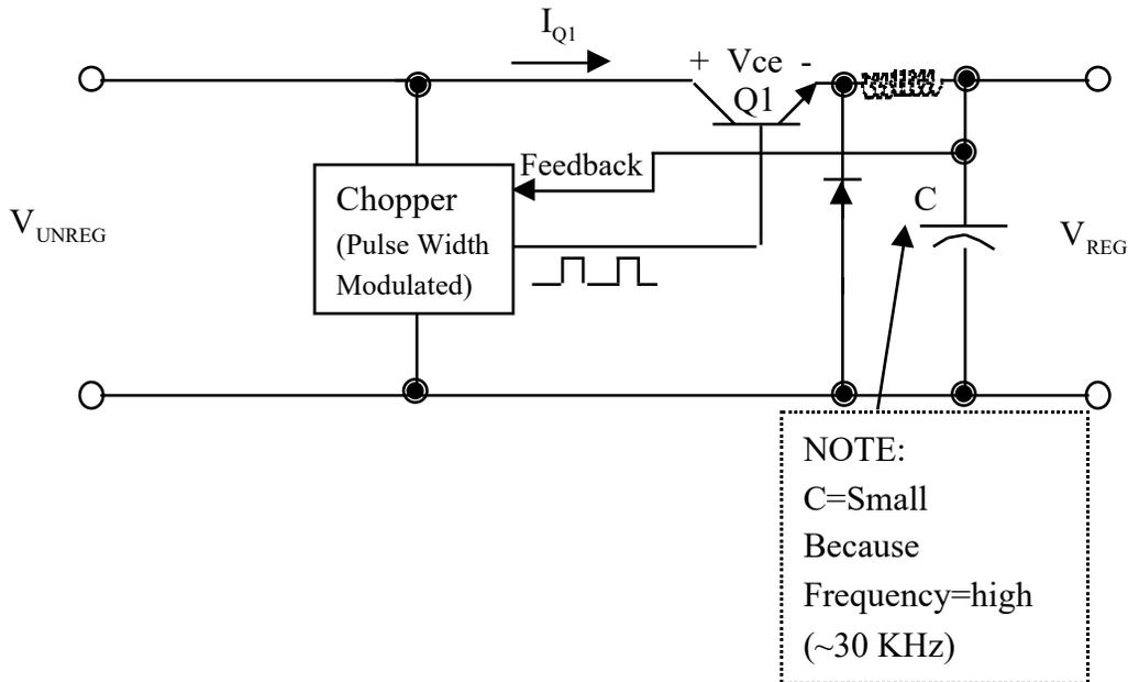
For the conditions:  $V_{UNREG} = 18 \text{ V}$ ;  $V_{REG} = 14 \text{ V}$ ;  $I_{Q1} = 1 \text{ A}$
