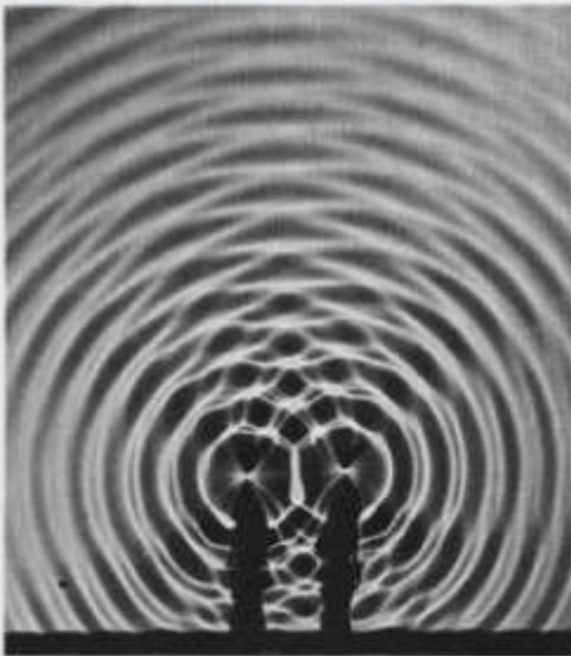
Figure 10-27. A photograph of the interference pattern of water waves from two point sources. Locate the nodal and antinodal regions.
